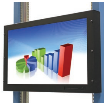
LTRM-423HD1 shown mounted in a standard 19" equipment rack.
